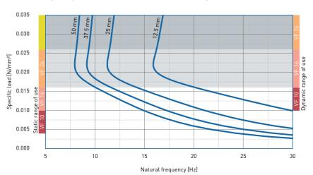
Natural frequency of a single-degree-offreedom system consisting of a fixed mass and an elastic bearing consisting of VIKAFOAM VF 16 on a stiff subgrade.
